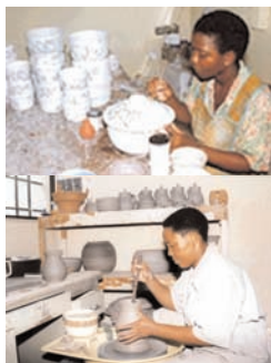
Body forming and decoration in ceramic technology
