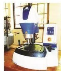
Polishing Machine for Polished Mount Preparation
